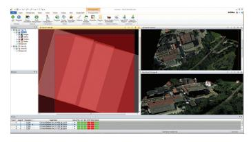
The very dense, very accurate RGB- or False-color-IR-encoded point clouds created with IMAGINE Auto DTM Semi-Global Matching have image-like quality and buildings with sharp, high-definition edges.
